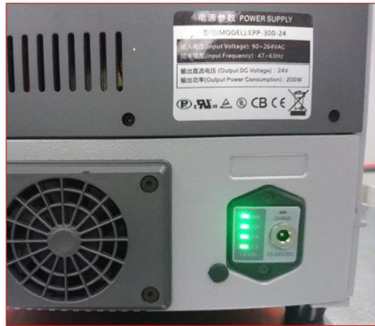
15 , The screen , LED , display of battery charger should be on after you press the emergency – stop button , if not ,check the connection again
