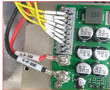
11, Fix the cable of 24V and cable of GND in the right position like picture show
