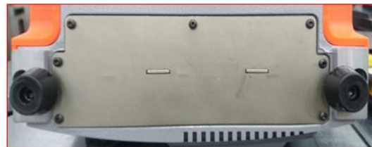
13, Fix the all cables after put back the mainboard , the mainboard should be in fixed very solid ,manage the cables again if not , then fix the foot rubber and screws
