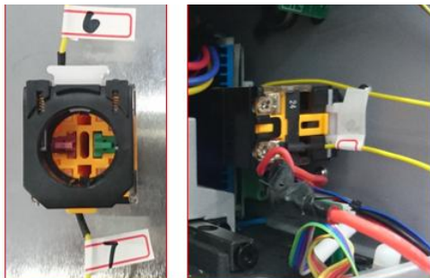
5, Fix the cable 6 to the position 12 , cable 7 for position 11 , then put the emergency – stop module back and fix it well
