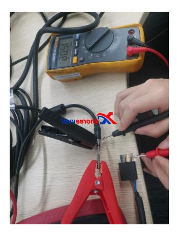
If the power is turned on and it cannot be continuously output 12V, or the power is turned off, there is still a 12V output, it means that there is a problem with the adapter and it needs to be returned to the factory for processing.
