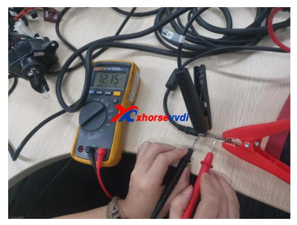
Now use the 12V on the platform to simulate the body battery. The black clip is the negative electrode of the body battery, and the red clip is the positive electrode.
