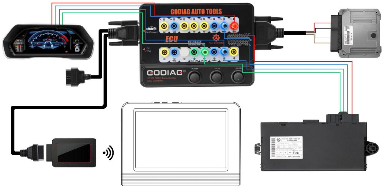
6. When to use the extension cables: The space of the diagnostic interface location is too narrow to connect to the diagnostic tool, or the user find that the diagnostic cable is not long enough during maintenance. It can be extended by 1.2 meters.
