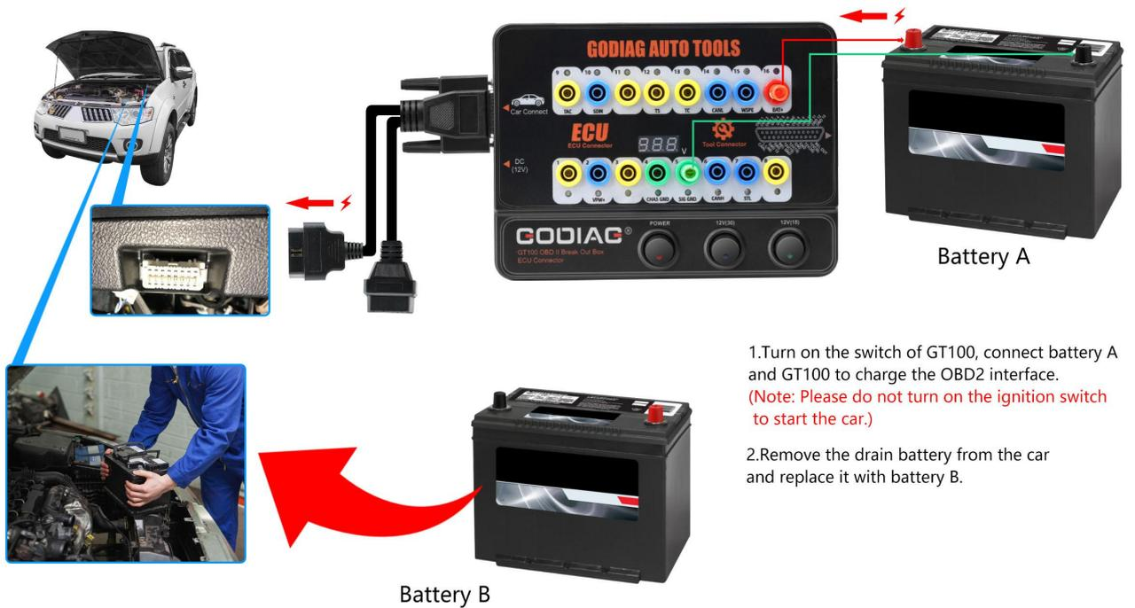
1). Prepare battery A to supply power by connecting to No. 16 / 4 / 5 holes of Godiac GT100 & to the OBD2 diagnostic interface of the car.
