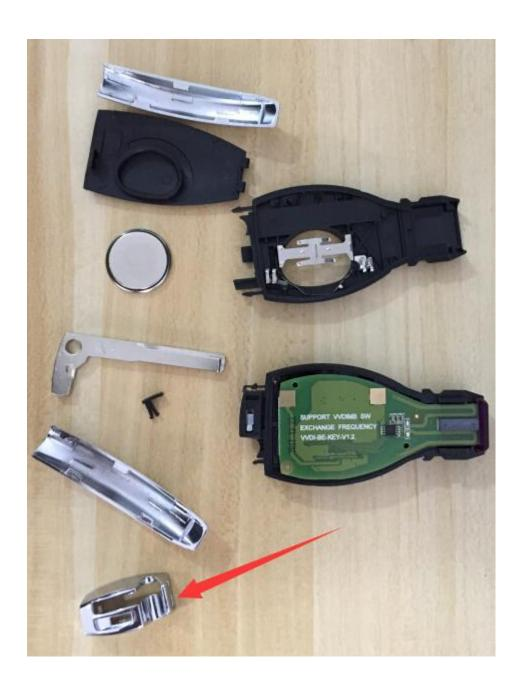
Note: If the rear metal component is firstly assembled, then the metal strips on both sides won't be able to put into the right position.
